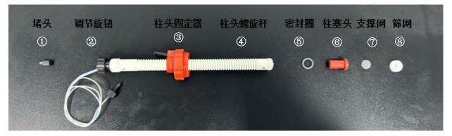
Note: ①plug②adjusting screw③adaptor fixator④adaptor screw rod
