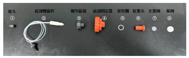
Note: ①plug②bottom screw rod③adjusting screw④bottom fixator⑤O-ring⑥column stopper⑦supporting mesh⑧sieving mesh
